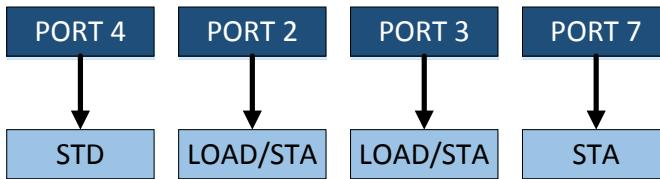
There are several execution units into one CPU core. These units are clustered around few execution ports
